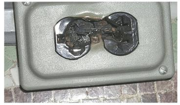
To the left is a burned and melted outlet found in a Congressional facility by the Office of Compliance on a fire safety inspection. This outlet is the result of electrical current overloading and an obvious safety hazard.
